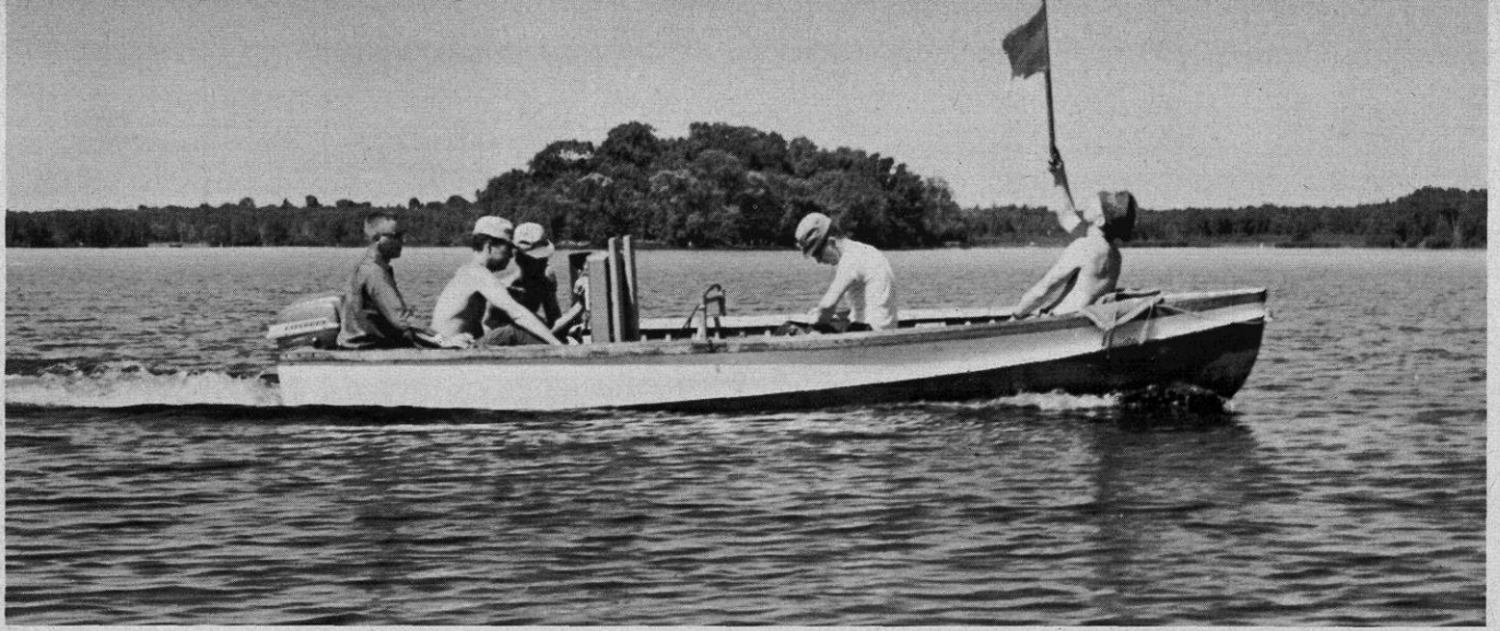
UW student civil engineers took part in hydrographic mapping of Lake Namekagon last summer. The flag is held aloft at pre-determined intervals to complete triangles with surveyors located on Namekagon Island, beyond the boat, and on the mainland at right. The box in the boat is a machine for recording depth readings obtained by sound probings.
