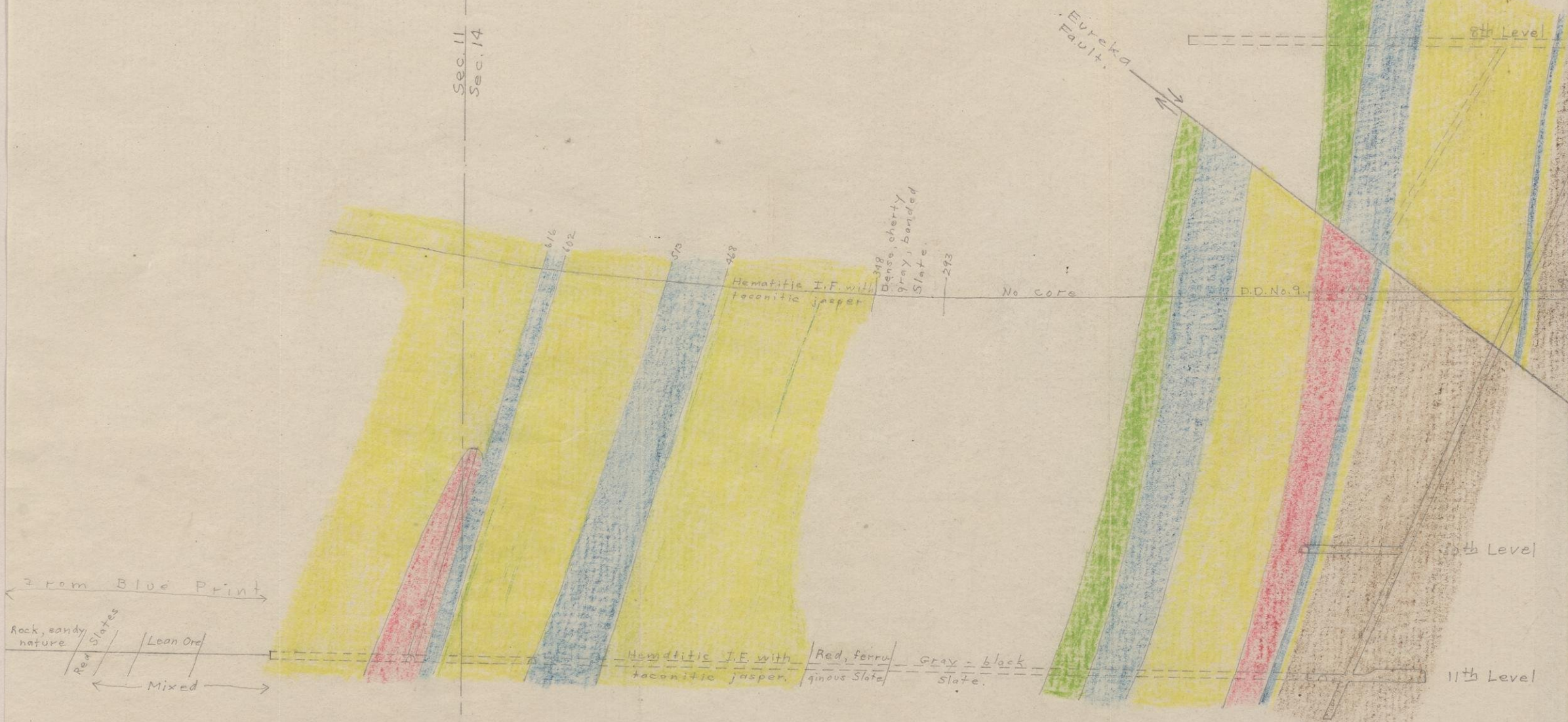
Section showing correlation of D.D. #9 and 11th Level Cross-cut. Anvil Mine Scale - 1" = 100'
