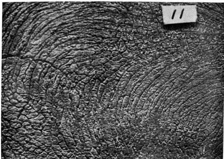
1. STEEL BURNED AND HARDENED (POLISHED). Magnified 2\frac{1}{2} diameters.
