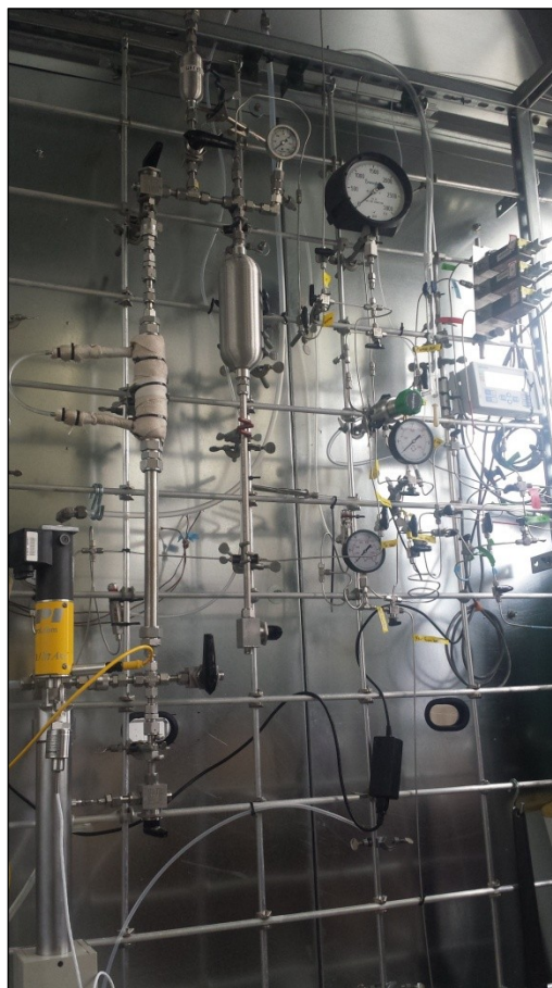
Figure 57. Schematic and photo of high pressure continuous slurry reactor for the production of fuels and chemicals from solid biomass derived compounds.
