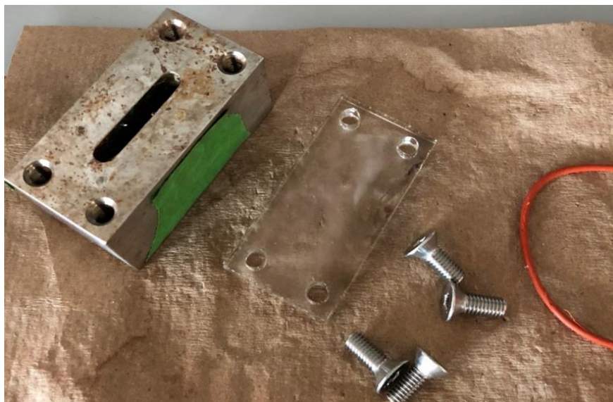
Figure 1: Diagram for the fabrication of a stainless-steel device for the formation of alginate hydrogels with internal architecture (top). The device contains inlet and outlet ports for needles to hold a tube molding material in place, an indentation in which an o-ring is held in place to seal an acrylic base in the bottom of the device, and ports for screws to hold the base in place (bottom).
