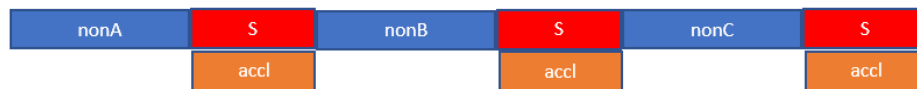
Figure 4.6: Frontend dispatch rate in the L_NT case. Although the TCA begins execution speculatively (no drain penalty), the CPU dispatch stalls until TCA completes execution.
