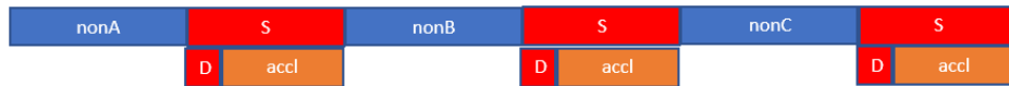
Figure 4.5: Frontend dispatch rate in the NL_NT case. Red denotes dispatch rates drop to 0 for either the CPU (top) or TCA (bottom) for stall (S) or draining (D) conditions. Commit penalties are considered part of the drain and stall penalties for graphical purposes.
