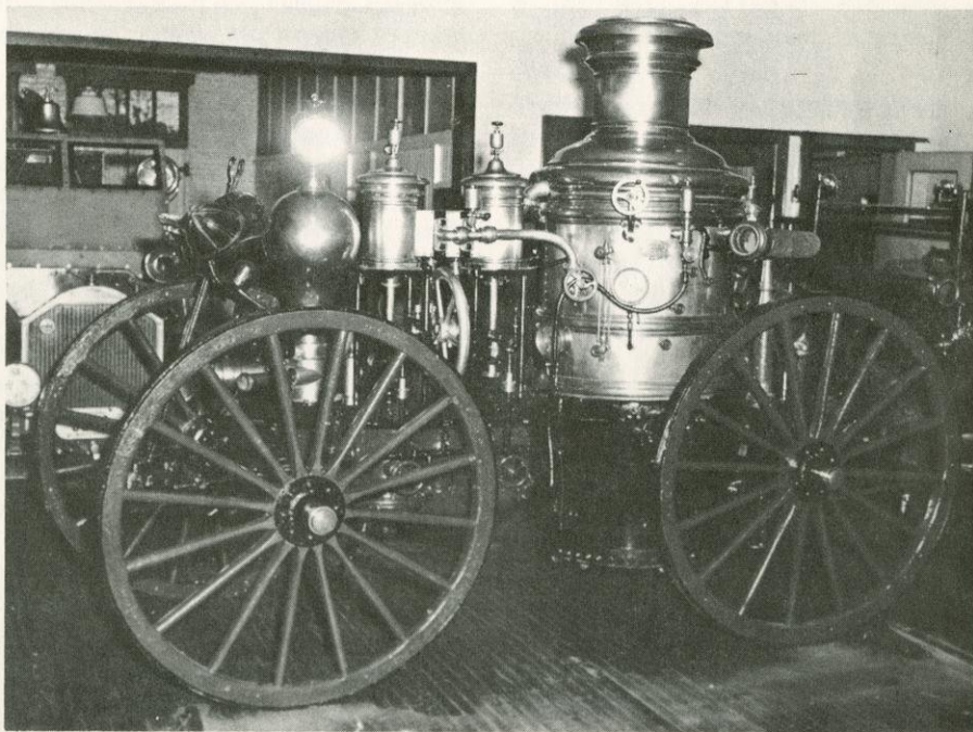
Water Tube Boiler made by American Fire Engine Co.
