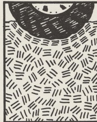
Don't run over your septic system drainfield during construction. The weight of heavy machinery changes soil alignment and restricts water flow.
