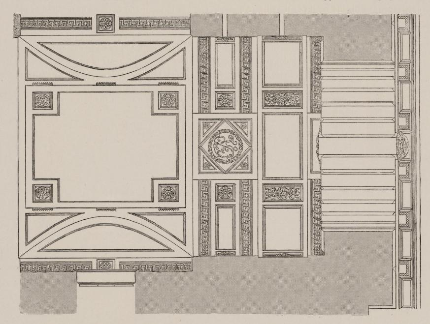
FIG. 7.—PLAN OF ARCHWAY LOOKING UP, SHOWING PART OF CEILING. R. W. Gibson dei.
