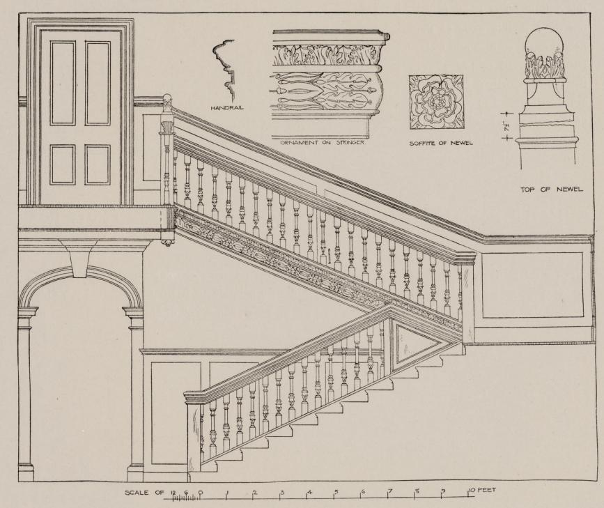
FIG. 26.—ELEVATION OF THE STAIRCASE. J. C. COOK del.
