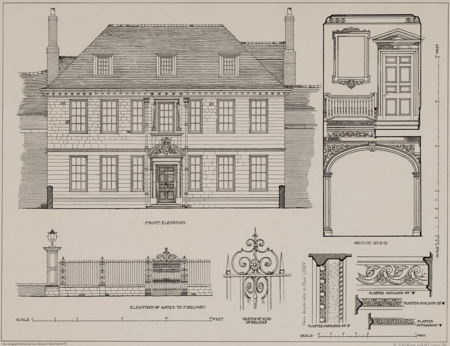
HOUSE IN THE CLOSE SALISBURY. ELEVATION WITH DETAILS OF STAIRCASE ETC.
