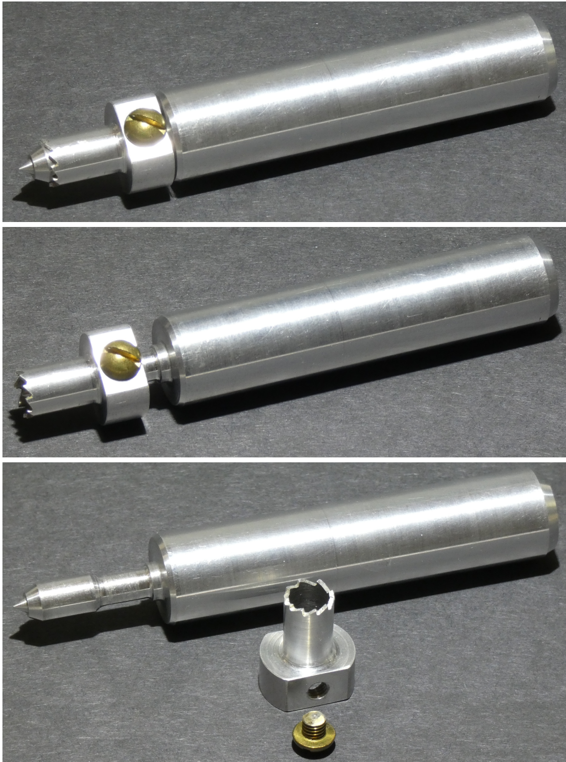
Figure 4.7: Tool for marking burr hole perimeter on swine skull. This marking tool consists of a pointed shaft with a captive sleeve that can slide along and turn about the shaft, all attached to a handle for easy manipulation.
