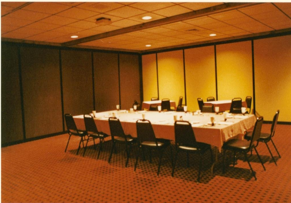
Portion of Scandinavian Room. Wall Dividers Move on Tracks to Create Various Sized Rooms
