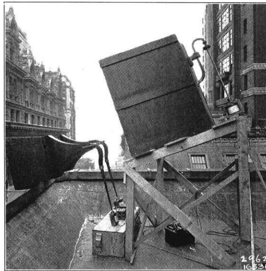
FIG. 1: Exponential Horn on the Westinghouse Building in New York City. Signals from it Were Audible for Many Blocks Along Broadway.
