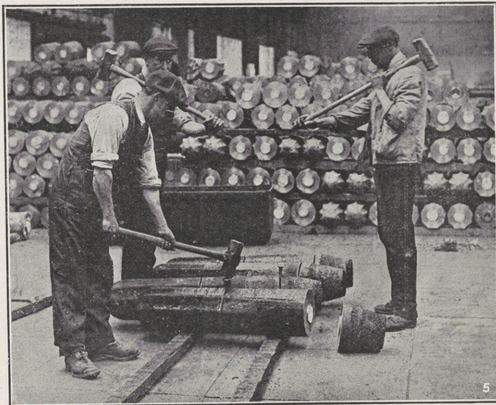
3. Loading Double Billets by Electric Magnets. 4. Double Billets for High Explosive Shell. 5. Breaking off Heads and Billets.
