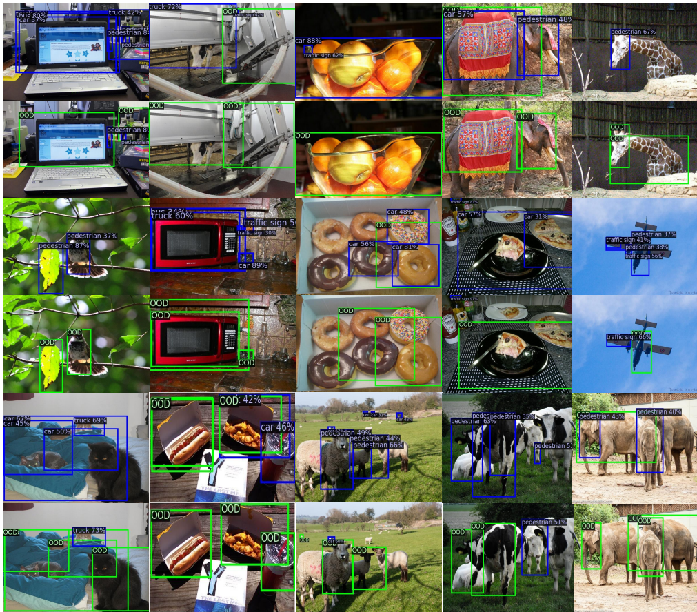
Figure 12.3: Additional visualization of detected objects on the OOD images (from MS-COCO) by a vanilla Faster-RCNN ( top ) and VOS ( bottom ). The in-distribution is BDD-100k dataset. Blue : Objects detected and classified as one of the ID classes. Green : OOD objects detected by VOS, which reduce false positives among detected objects.
