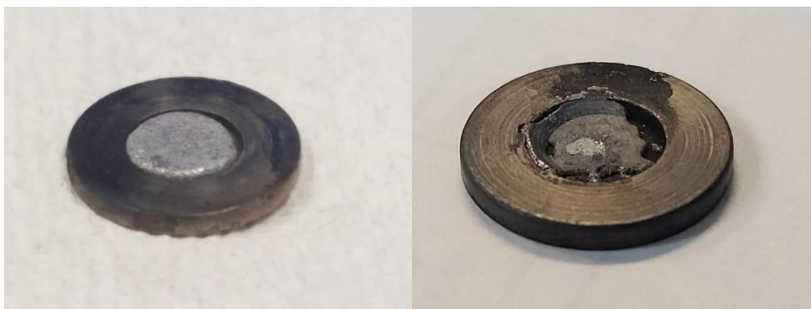
Figure 13: A thick ( $\sim 460$  mg, **left**) and a thin ( $\sim 185$  mg, **right**), unmilled  $\text{CoGa}_2$  target after hot-pressing into the niobium crucible.
