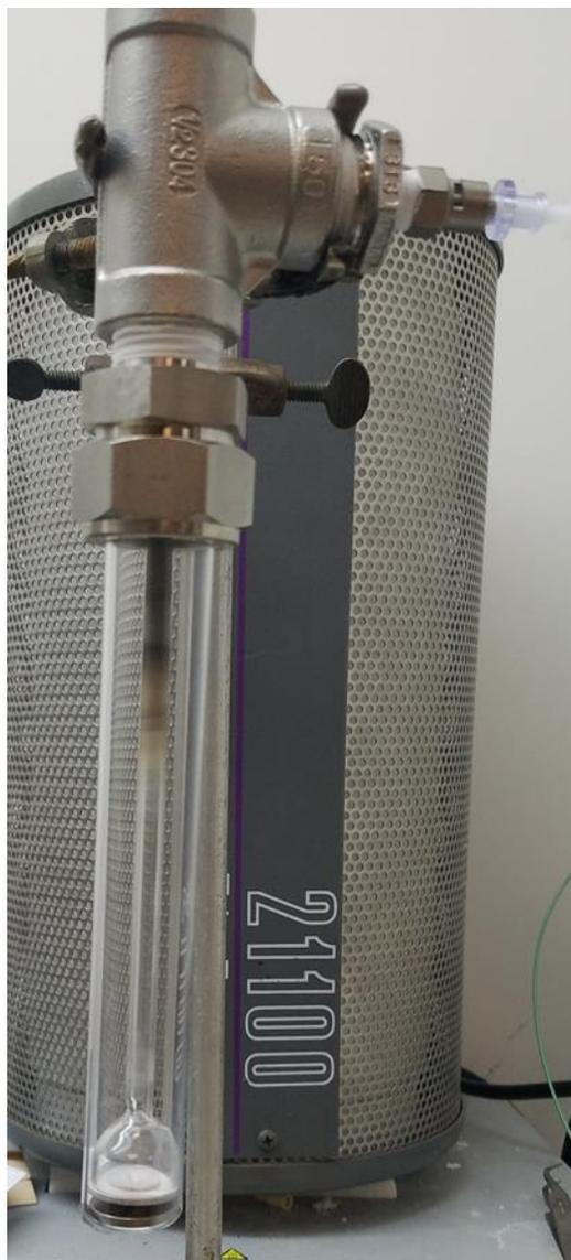
Figure 12: The hot-pressing rig with niobium crucible,  $\text{CoGa}_x$  pellet, boron nitride tamper, and bell-ended quartz glass rod for pressing and gas flow egress (bottom to top)
