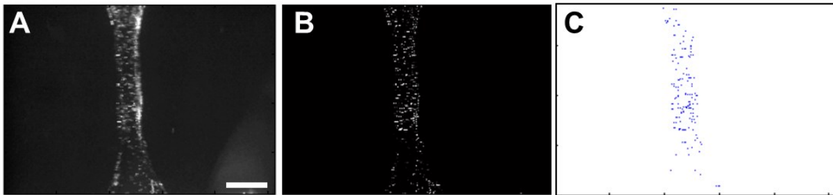
Figure 2-2. Quantification of particle locations, conducted using track.m software developed by John C. Cocker of University of Pennsylvania. Raw images (A) are first filtered to improve the accuracy of particle detection (B). Once particle locations are quantified, they are plotted during analysis (C) to allow the user to observe the accuracy of the particle tracking software. Scale bar = 2 mm.
