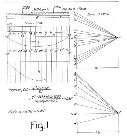
The following notation will be used to determine the deflection of the beam:
