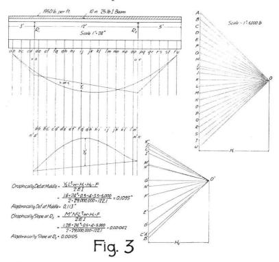
For deflections of the overhanging ends, the moment of the bending moment area will be involved as in the case of a cantilever, but here must be taken into consideration the fact that the slope at the two supports is not zero. As shown in Figure 3, the slope at the supports is proportional to the reaction at each support as determined by the second force polygon in this figure.
