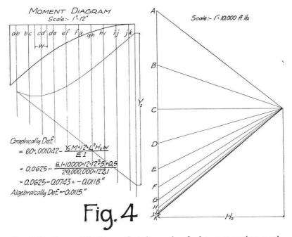
the deflection. We know that in a simple beam treating positive bending moment area as a downward load on the beam we would get upward or positive reactions and the slope at the right support would be positive. So if on this basis the reaction at the right support is positive we know the slope is positive. Conversely, if positive moment is treated as an upward force, then the reaction at the right support would be negative, and then negative reaction would mean positive slope.
