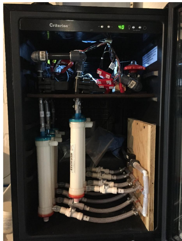
Figure 17. Photos of both automated sampler designs. Sampler 1 (on left) is labeled to show the location of the YSI EXO sonde containing the water-quality sensors, the datalogger and the four hemodialysis filters. Sampler 2 (on right) holds eight filters and is contained within a small refrigerator. The datalogger (not in the picture) sits on top of the refrigerator.
