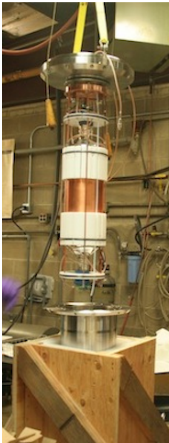
Figure 4.7: Prototype being placed into pressure vessel at Physical Sciences Laboratory
