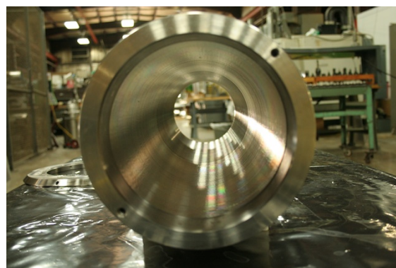
Figure 4.4: Stainless Steel Pressure Vessel. A pressure vessel is needed to protect DM-Ice17 from the high pressures during refreezing in the ice after deployment.
