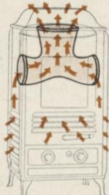
The exclusive Intensi-Fire Air Duct—the heart of Heatrola's double air-circulating system. This ingenious device greatly increases Heatrola's heating capacity by capturing and utilizing heat that in ordinary heaters goes to waste up the flue.
