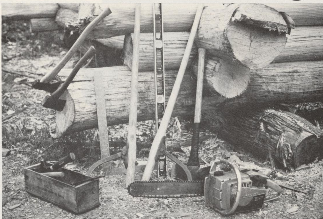
Log builder's tools: hand axes, builder's square, cant hooks, board or hewing axe and chain saw. Smaller tools including wood scribes, compasses, and other items are in the small box. Photo by author.
