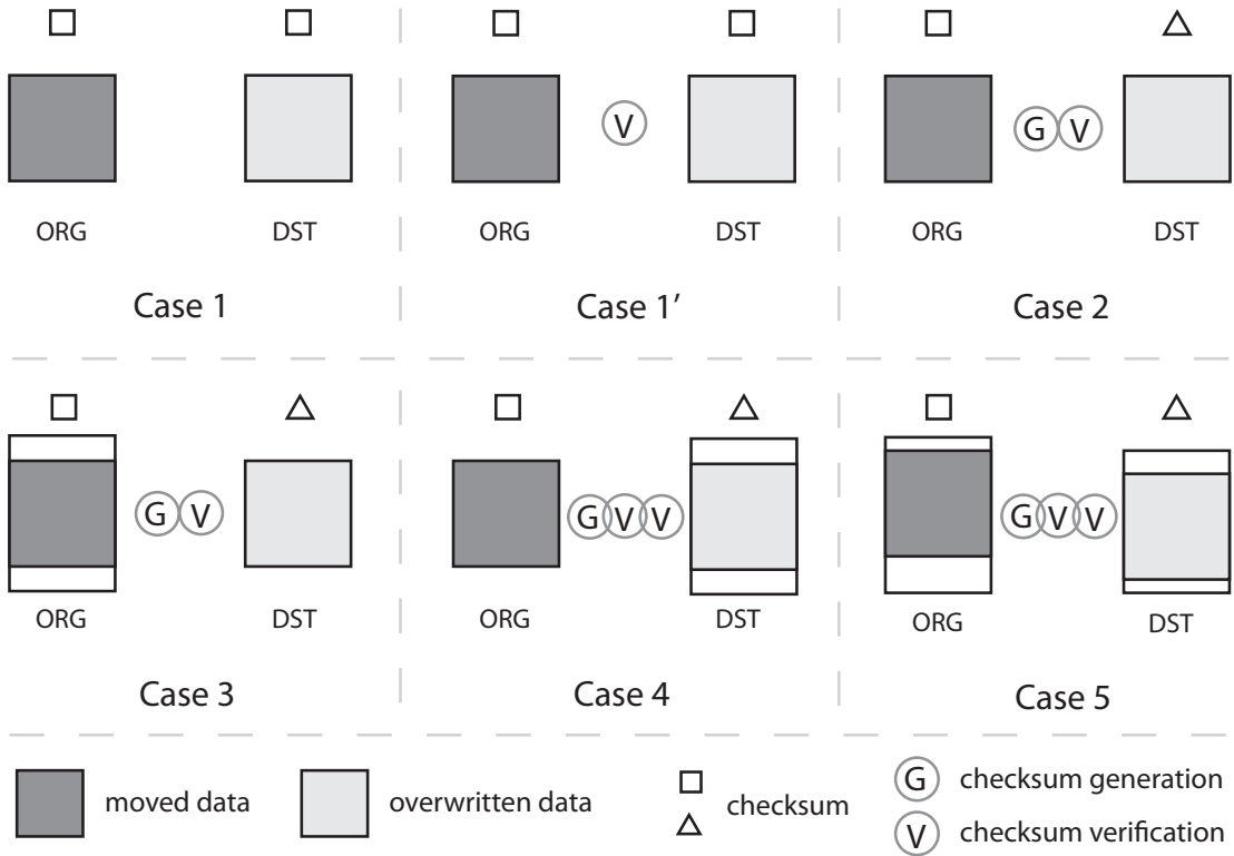
Figure 4.14: Cases of Checksum Chaining This figure shows five typical cases of data movement. In Case 1, 1' and 2, the moved data is aligned with ORG and DST . In Case 3, 4 and 5, the moved data is not aligned with ORG , DST or both, respectively. The size of moved data could be the same as DST.size as in Case 1, 2 and 3, or different as in Case 4 and 5. The sequence of checksum chaining is shown as G and V operations in each case. The number of these operations is used as an estimate of the overhead.
