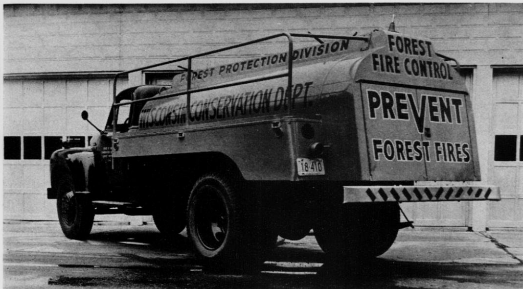
The trunk-tank unit shown here is among many items the Conservation Department has acquired from the federal government, and converted to forest protection equipment at very reasonable cost.
