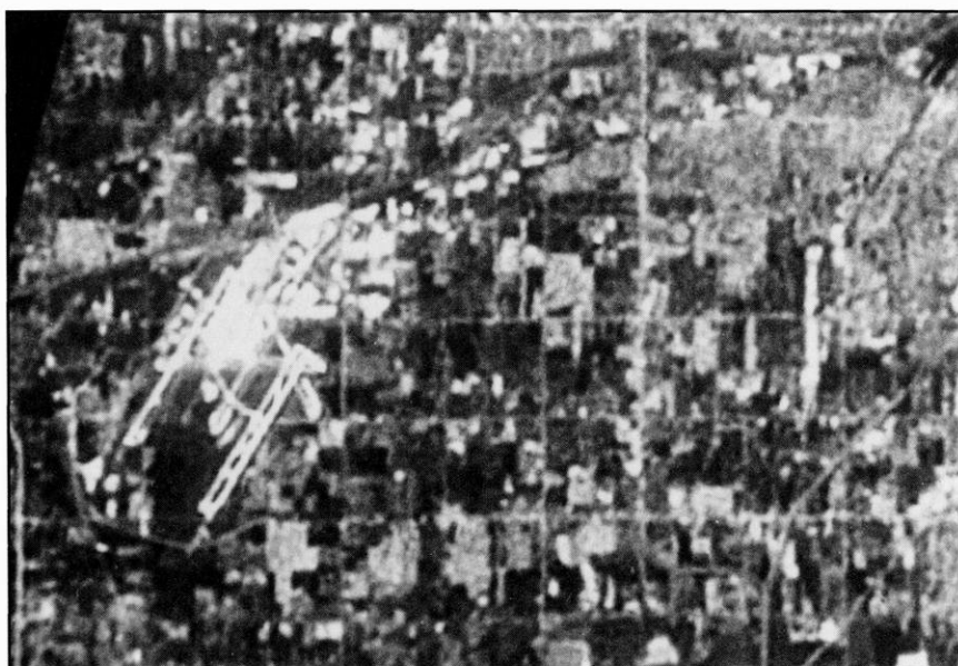
FIGURE3. Detroit airport and vicinity imaged by Landsat-3 multispectral scanner (MSS) from a height of 900 kilometers.
