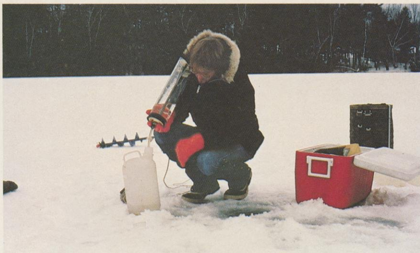
Water samples taken year-round are tested for buffering capacity, pH and other chemical components. Photo by Joe Eilers
