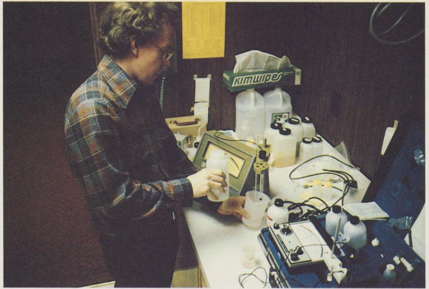
Researcher Ron Becker tests the pH of precipitation at the DNR laboratory at Rhinelander.
