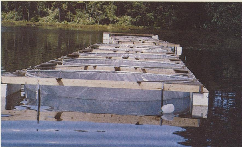
Acid will be added to each compartment of these "limno-coralls" to determine how different amounts affect the biota. Photo by Dave Kunelius.
