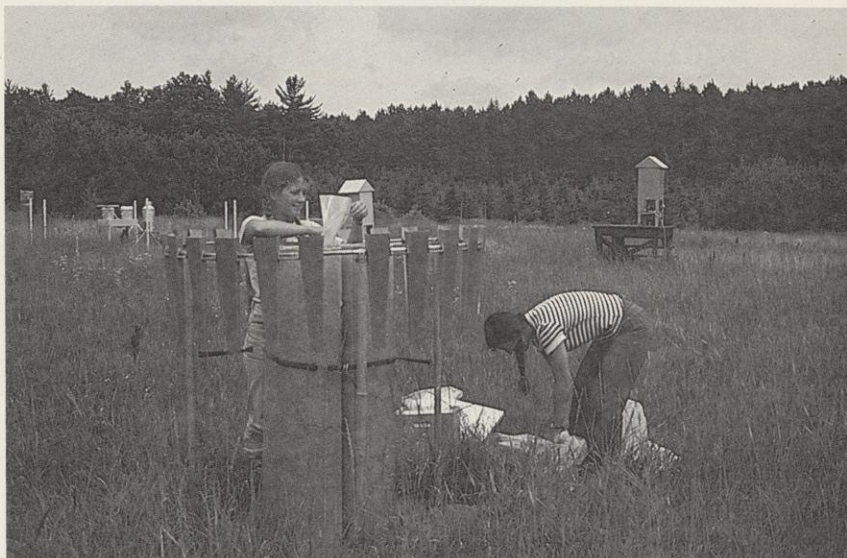
Bags that contain deposition at Trout Lake are changed every 30 days and sent for analysis. Here Lisa Huberty and Nan Eckert of DNR's acid rain research team make the switch. Photo by Katherine Webster
