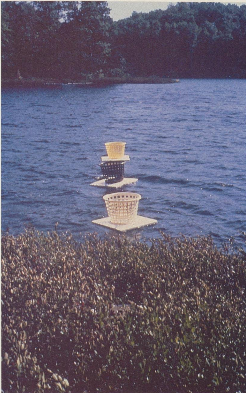
About 40 laundry baskets were floated on the lake to collect leaves and other material that falls into the water for analysis. Photo by Katherine Webster
