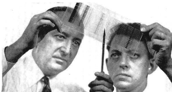
At Great Lakes Steel a spectrogram is readied for reading in the densitometer—one of the tests that assure quality steel.
