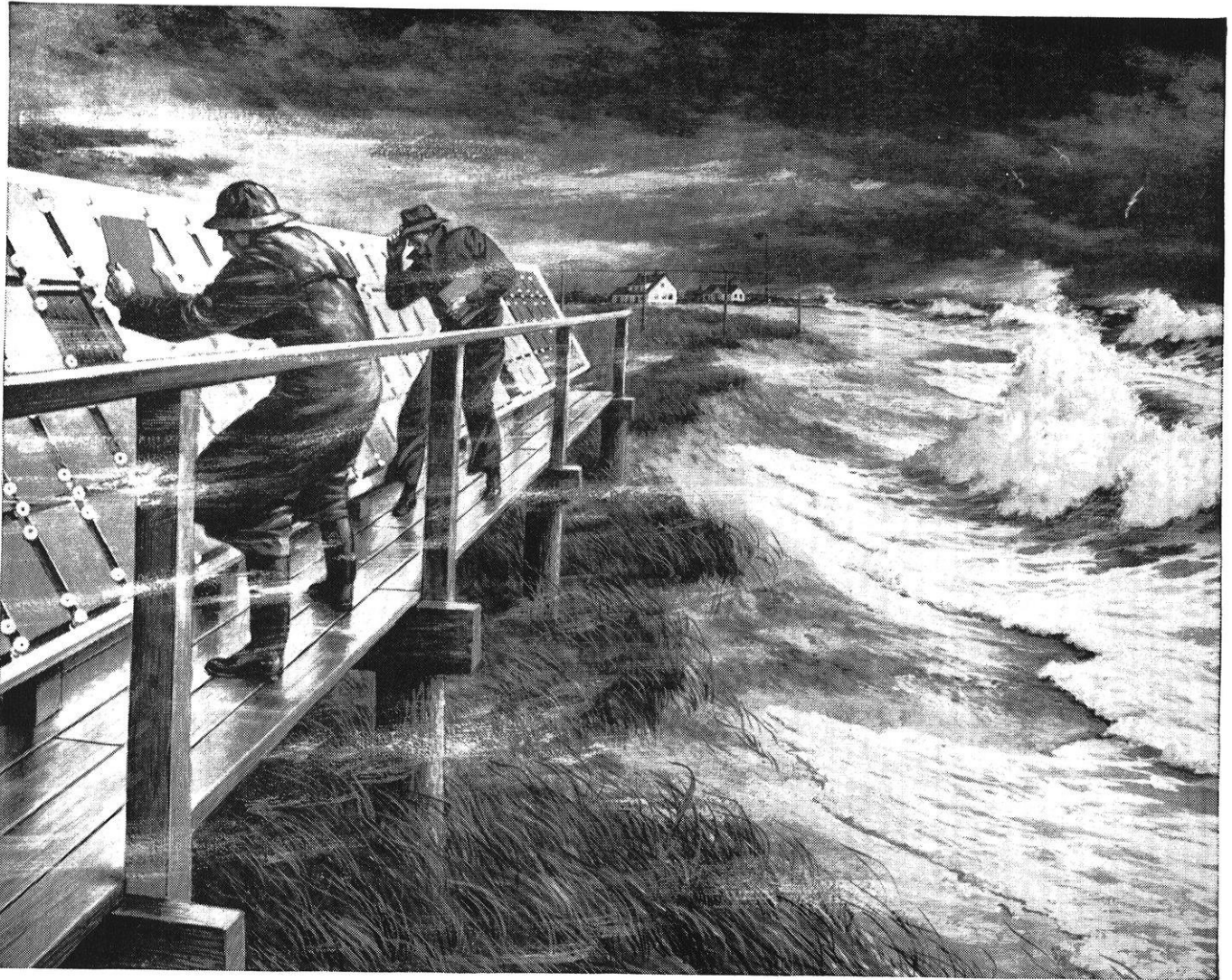
Ocean Laboratory —here at its big Kure Beach, N. C., Testing Station, Inco exposes thousands of metal specimens to the corrosive effects of salt spray, salt air, salt water.
