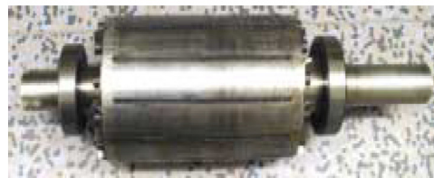
Fig. 1.37 Cross-sectional view of a memory motor and its rotor prototype [107, 108]
