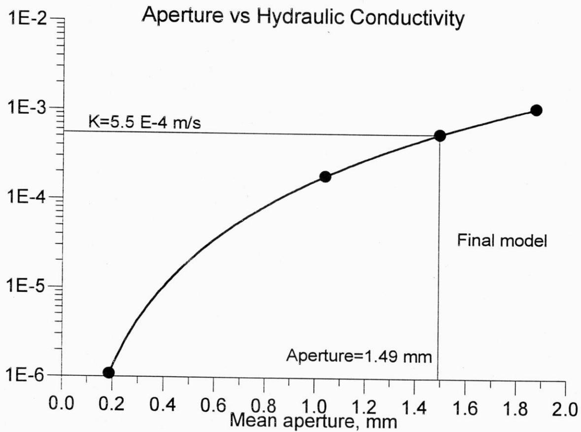
Figure 8. Mean aperture versus hydraulic conductivity for the Door County data.
