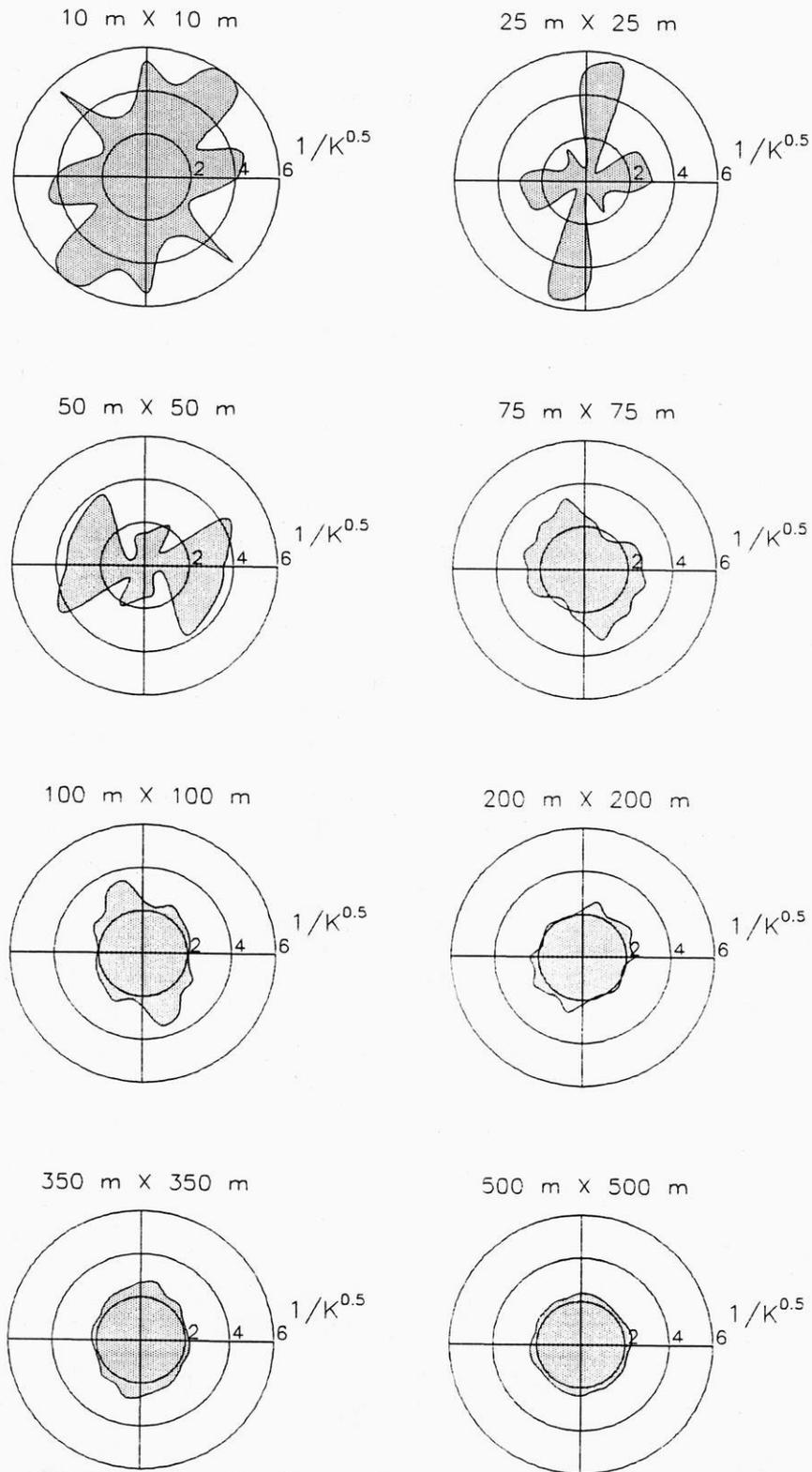
**Figure 6.** Plots of directional hydraulic conductivity (m/s) computed using the SDF model at various problem scales.
