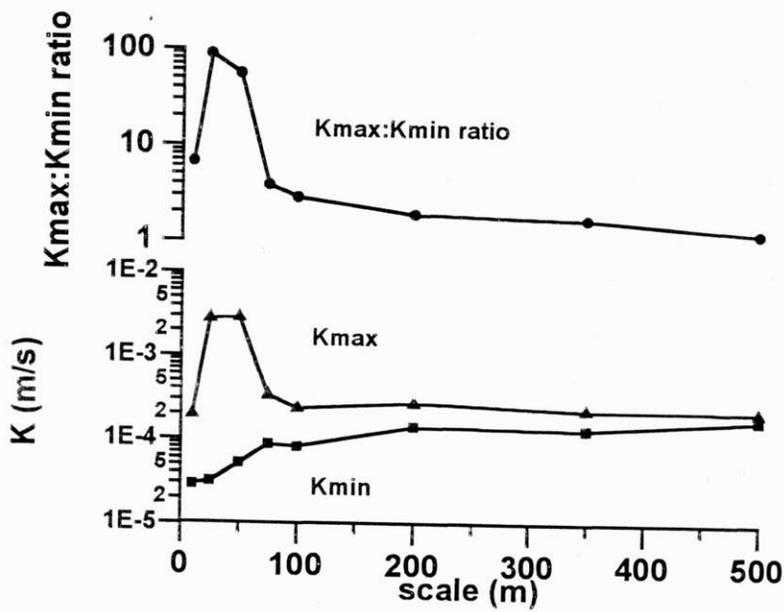
Figure 7. Minimum and maximum directional hydraulic conductivity and the  $K_{min}:K_{max}$  ratio versus scale of the problem for fracture simulations based on the Door County data.
