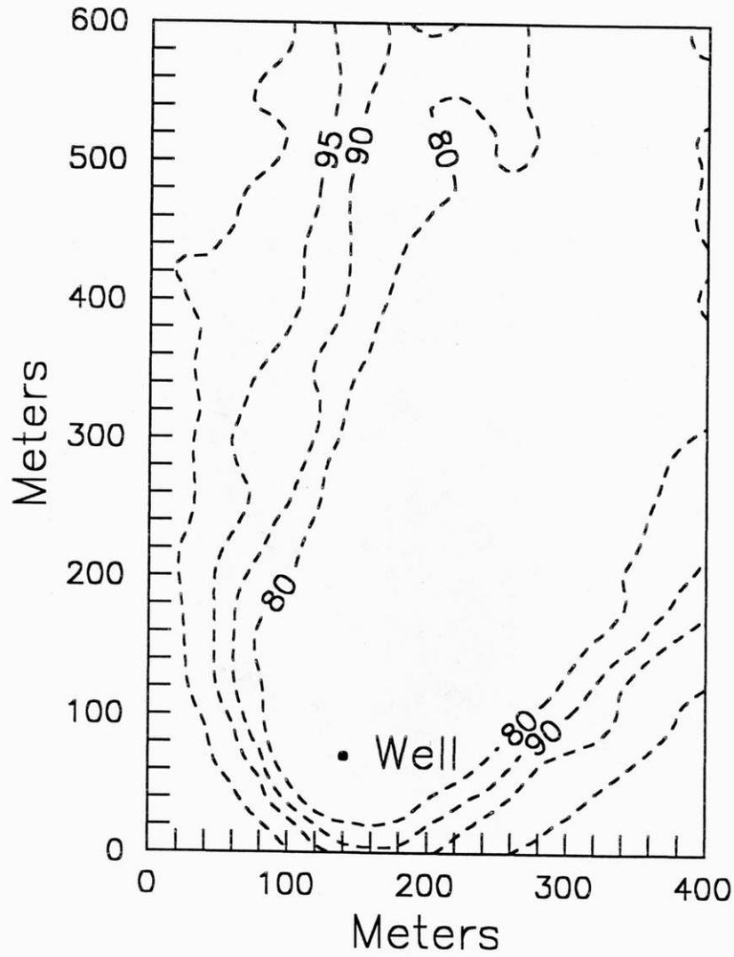
**Figure 11.** Percentage of particles captured in space for the SDF model simulation shown in figure 10.
