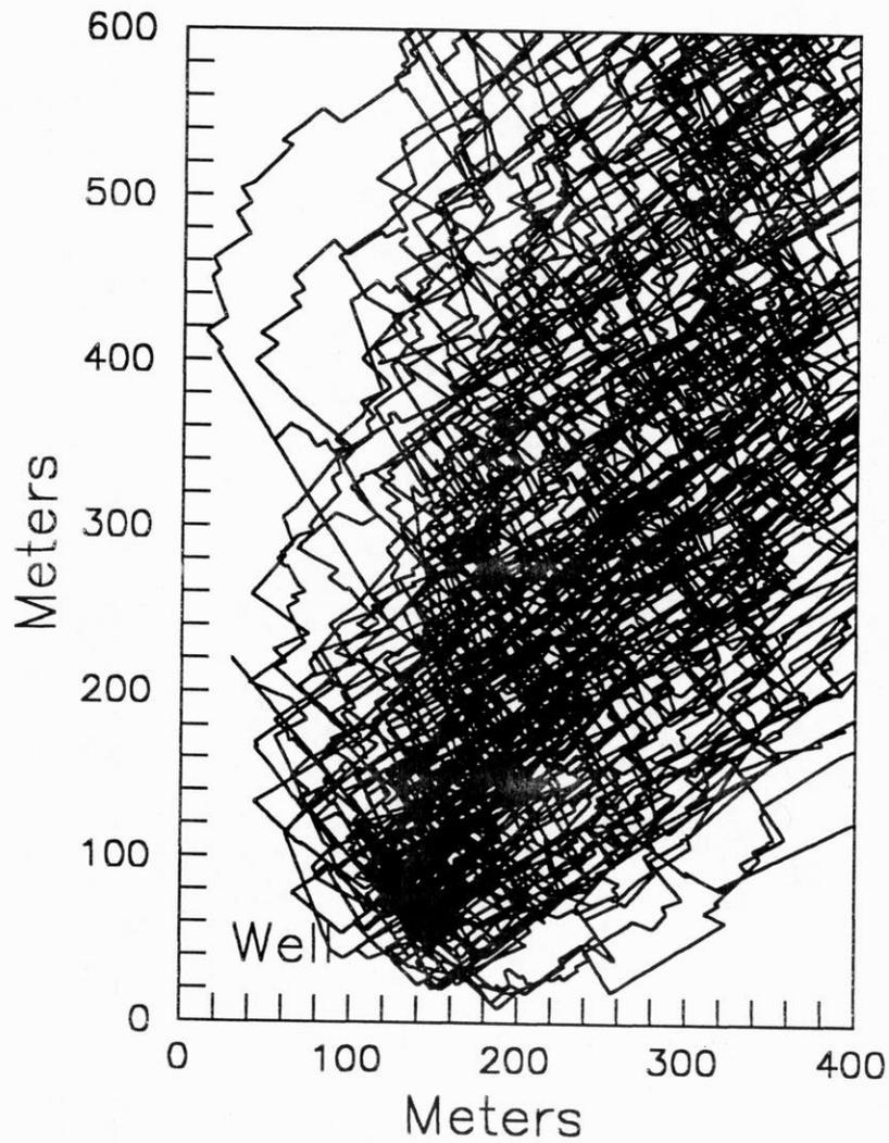
**Figure 10.** Particle paths for the SDF capture zone experiment in the same domain as figure 9. The plot represents 20 realizations of 10 particles each.
