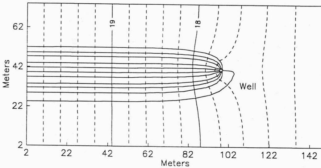
**Figure 4.** Particle paths from an upgradient boundary (left side) to a steadily pumping well in a uniform porous medium.
