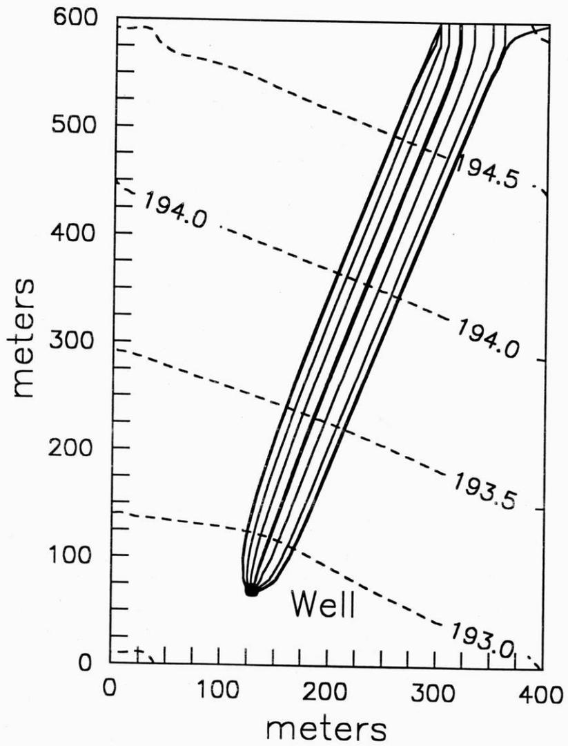
**Figure 9.** Capture zone for the Door County field site delineated using a porous-media model. Equipotential lines show simulated hydraulic head in meters above mean sea level.
