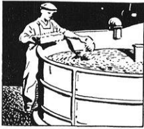
High quality wood pulp now used to form a sleeve around the wire
