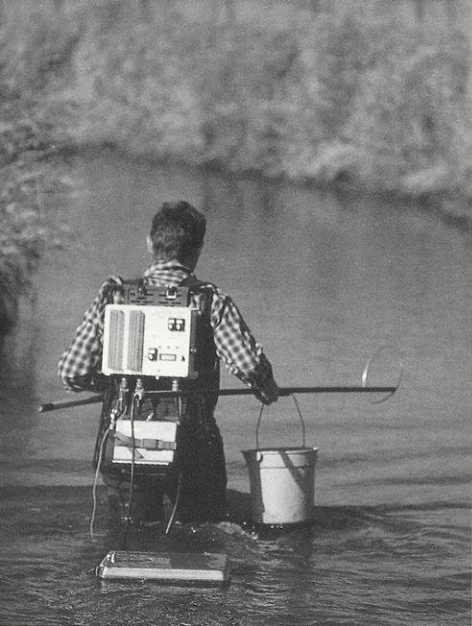
Sampling water chemistry and surveying the aquatic population to measure if this trout stream is still healthy.
