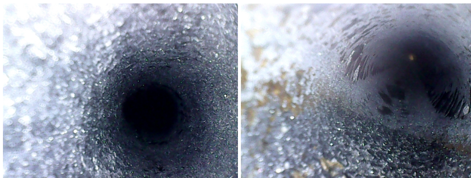
Figure 6.7: The top cross entrance (Left) and exit (right) showing a layer of metallic crystals.
