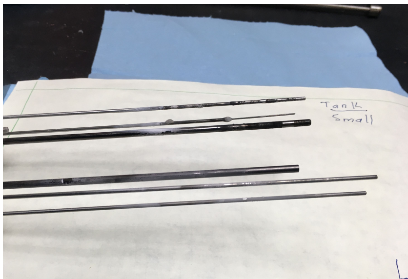
Figure C.10: First generation electrochemistry probes showing the depleted molybdenum electrode from the small tank.
