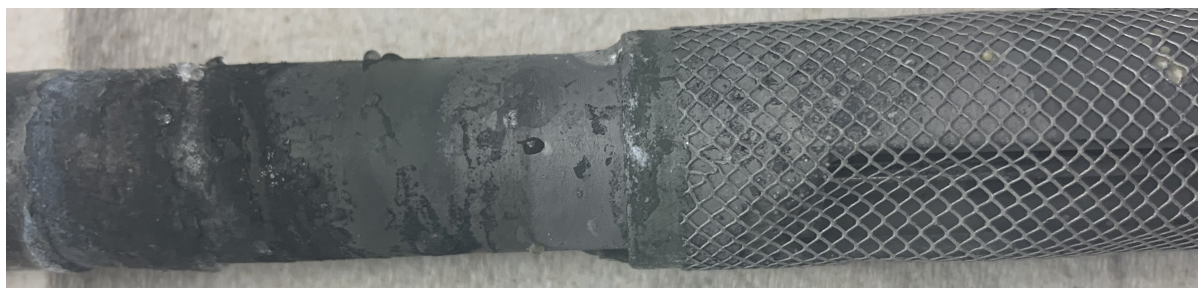
Figure C.11: Second generation electrochemistry probe with a nickel mesh that appears unaffected by the salt compared to the darker stainless steel tube.
