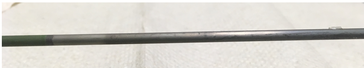
Figure 3.16: A stainless tube showing the green coating in the gas space compared to the matte color for the salt-wetted section.
