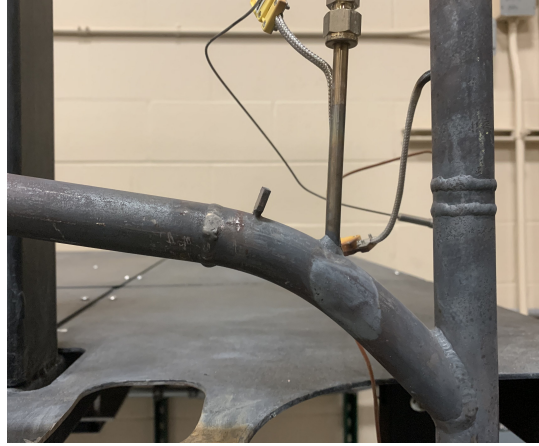
Figure C.4: The loop metal survived the blow torch test with minor discoloration.
