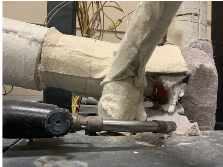
Figure C.3: A temporary gap in the insulation for time-of-flight measurements using transients generated with a blow torch.
