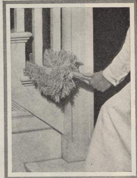
This dust mop is made of strands sewed to a canvas bag, which is shaped like a two-tined fork. The bag is slipped over a wire frame of the same shape and tied to the wooden handle with tapes. Its form makes it excellent for dusting banisters of stairs and the rounds of chairs.
