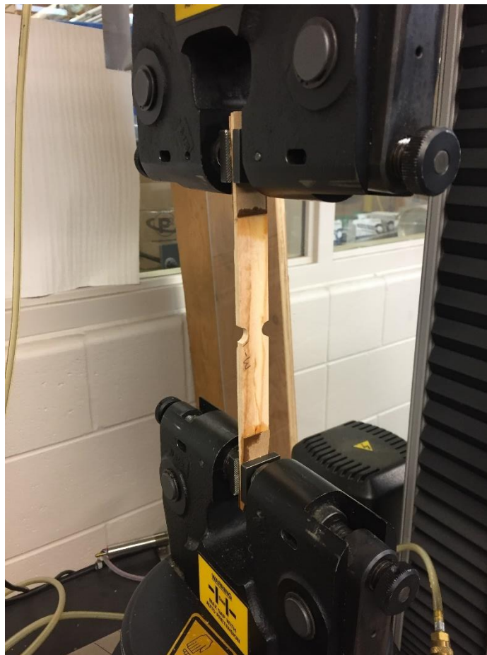
Figure 7-16: Loaded specimen in Instron tensile machine at 0.15 cm/minute.
