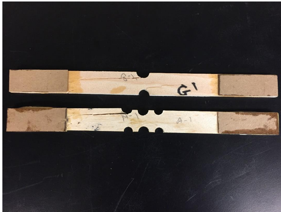
Figure 7-18: Failed Sitka Spruce specimens.
