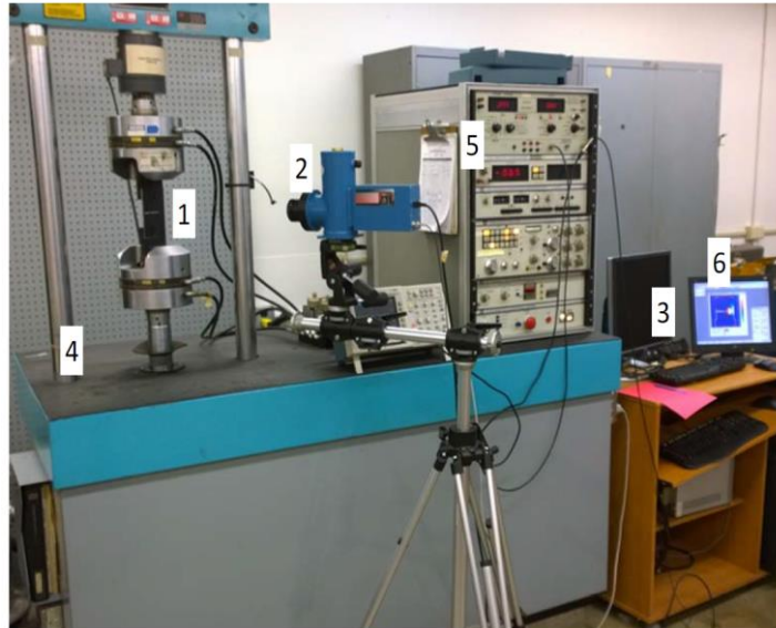
Figure 5-13: Experimental test setup for recording temperature variations of (1) finite plate with U-notch using (2) Delta Therm model DT1410 infrared camera, (3) computer to analyze image data, (4) load frame, (5) servo-hydraulic testing machine control panel, and (6) TSA image of loaded specimen.
