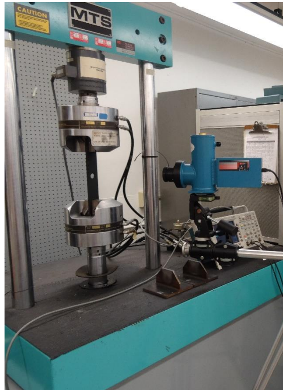
Figure 3-15: Experimental test setup for recording temperature variations of finite plate with elliptical hole using Delta Therm model DT1410 infrared camera.
