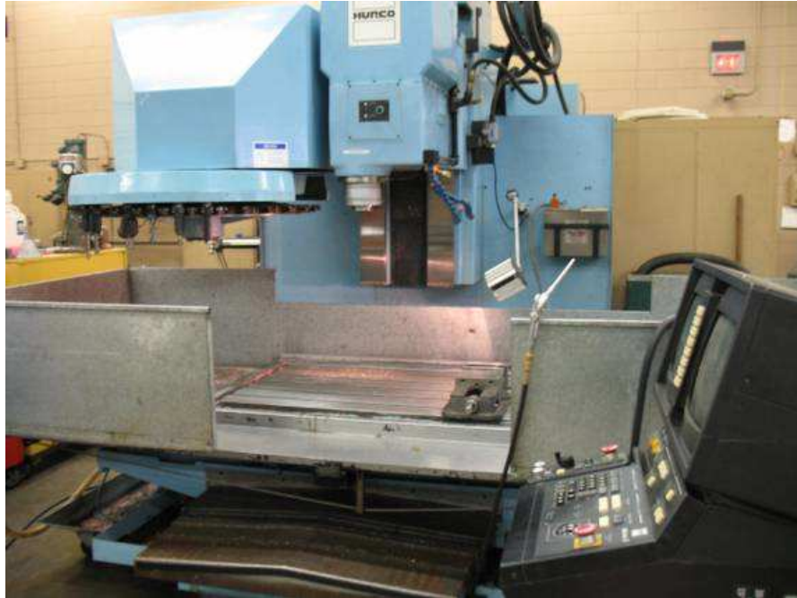
Figure 3-3. 15hp Hurco BMC 40 CNC machining center used for this experiment
