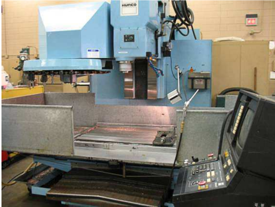
Figure 4-4. 15hp Hurco BMC 40 CNC machining center used for this experiment
