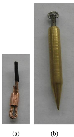
Figure 5.39: (a) Prototype eye-loop like those placed at the bottom of each ‘double-strength’ TTT calibration source. On each final source, a small split ring was strung on the eye-loop for attachment to the brass weight. (b) Brass weight for ‘double-strength’ TTT calibration sources.
