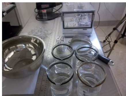
(b) Beakers of pieces in the clean room, just before being drained following final rinse. The bowl and sieve used for draining are visible, as is the previous batch of copper pieces drying in petri dishes inside the desiccator cabinet in the background.
