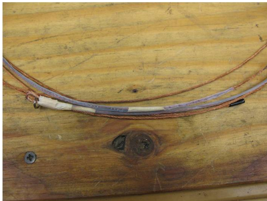
Figure 5.40: A completed ‘double-strength’ TTT calibration source. The taped wire ends are visible under the PTFE tubing, and the split ring can be seen on the eye-loop.
