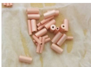
(a) Copper pieces after being drained following cleaning in acid solution.
