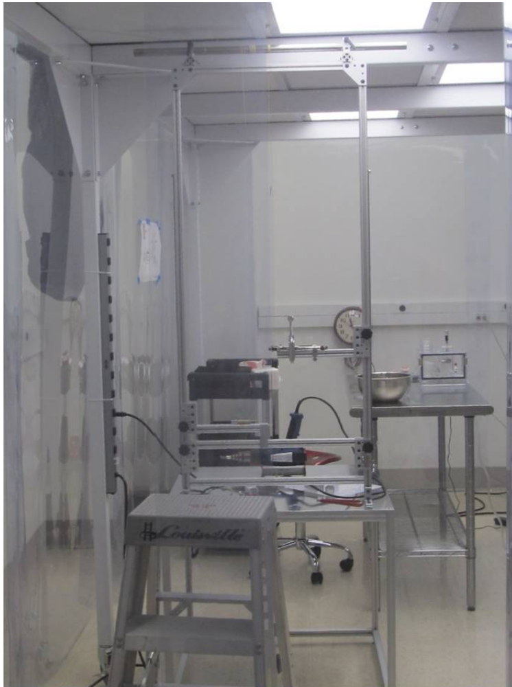
Figure 5.34: A photograph of the final source carrier jig in the UW clean room. A spacer can be seen positioning the pliers arm, and the heat gun in its stand is visible behind the jig frame.
