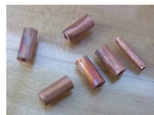
(c) Discoloration of copper pieces visible after drying.
