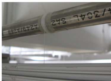
(b) The non-active Kevlar is stored on the top pipe during source carrier assembly.
