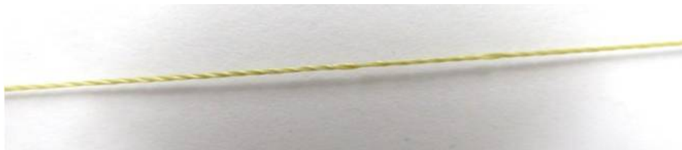
Figure 5.20: Photograph of PTFE-coated Kevlar after prolonged ( \approx 3 minutes) exposure to heat gun. Discoloration is less pronounced than that observed on silicon-wax-coated Kevlar after similar exposure (cf. Figure 5.30). Photograph from J. Clark.
