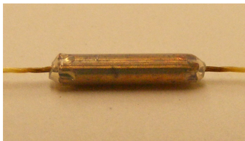
Figure 5.8: A photograph of a completed prototype source capsule. The darkening of the silicon-wax coating of the string is due to the heat used to shrink the PTFE sleeve.
