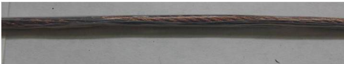
Figure 5.38: Close view of part of the active region of a ‘double-strength’ source produced for the high-rate calibration test in the Three Towers setup.
