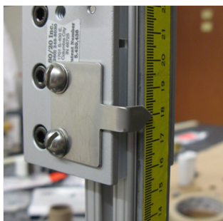
(a) Each side rail is marked with a scale in units of millimeters, and each end of the main reference bar is equipped with a pointer for alignment at predefined capsule positions.
