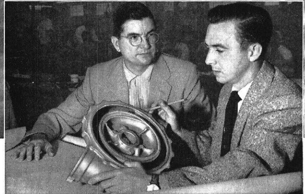
AiResearch two stage lightweight gas turbine compressor provides pneumatic power for aircraft main engine starting and serves as auxiliary power source for a variety of ground and in-flight services.
