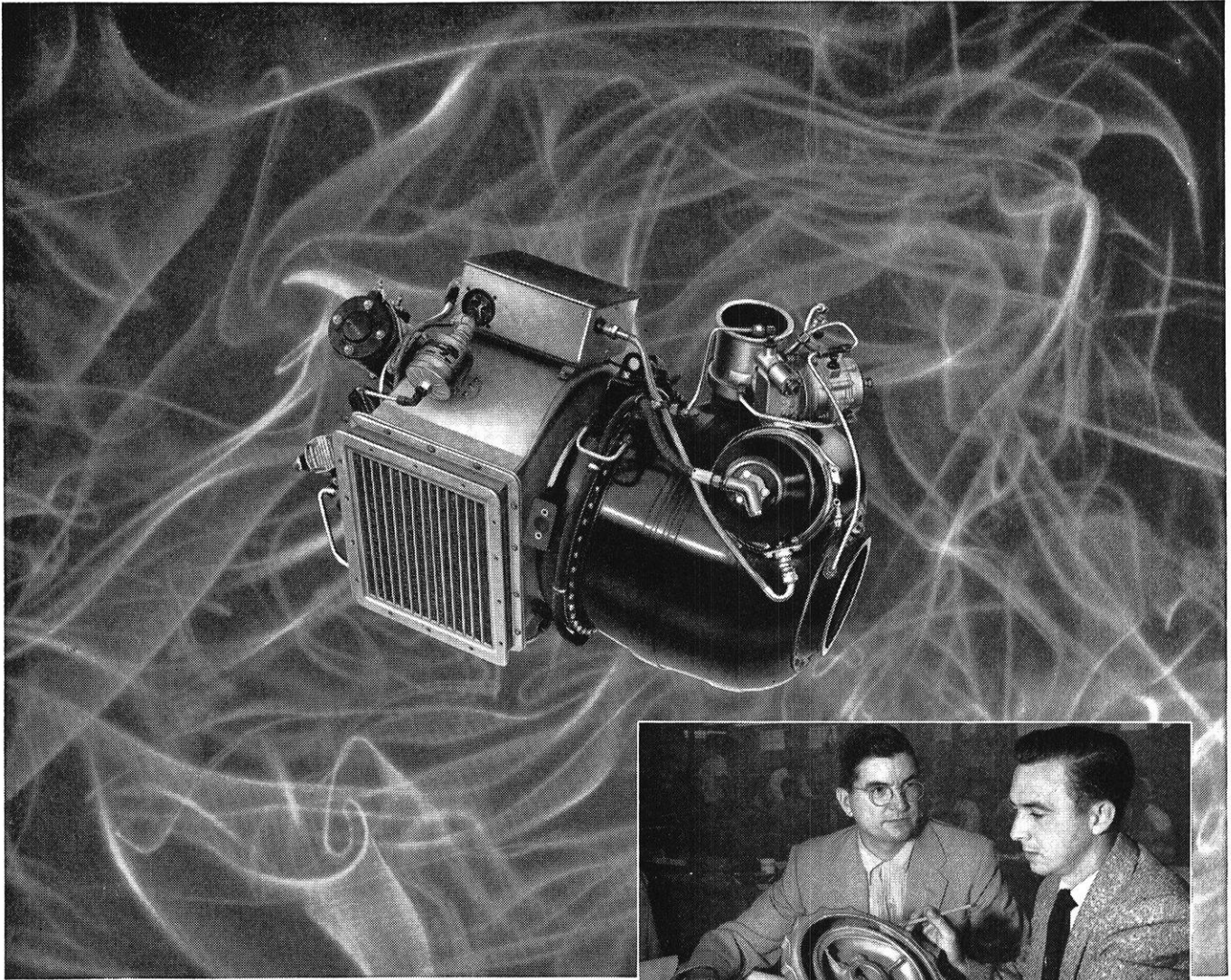
AiResearch two stage lightweight gas turbine compressor provides pneumatic power for aircraft main engine starting and serves as auxiliary power source for a variety of ground and in-flight services.
