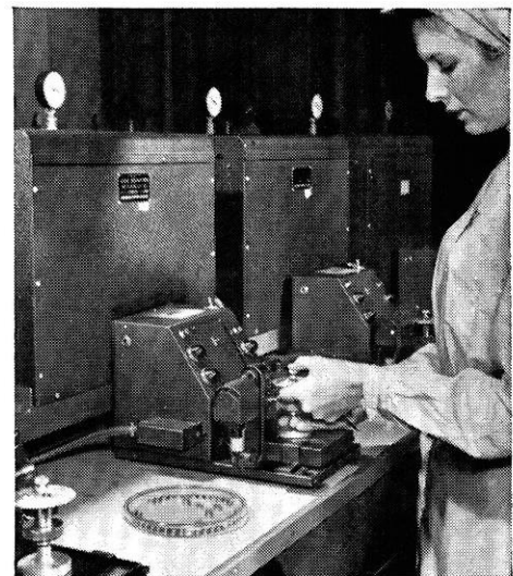
Automatic gram-centimeter torque tester measures starting torque characteristics of New Departure instrument ball bearings. Like many of the ultra-precise devices used in bearing manufacture, this torque tester was largely developed by New Departure.
