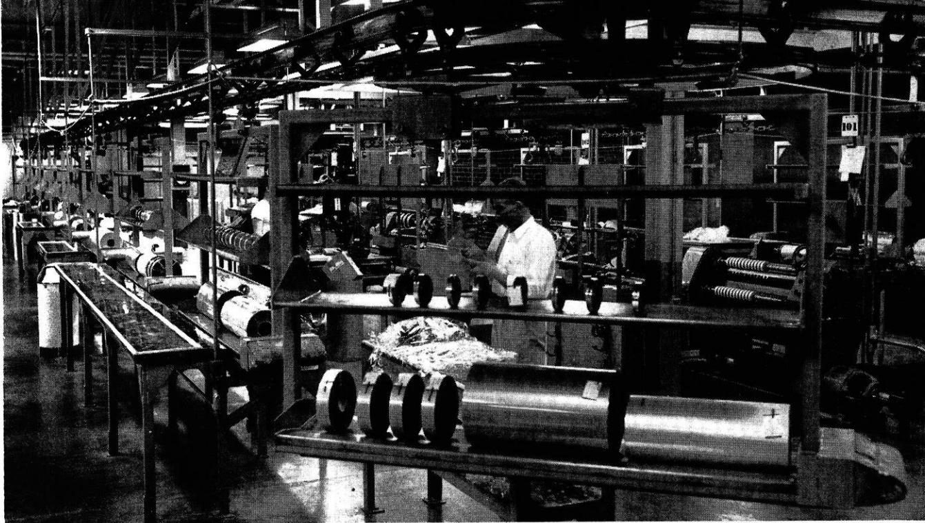
Du Pont's new "Mylar" polyester film emerges in a continuous sheet at the end of the manufacturing at the Circleville, Ohio, plant. It is then wound on large mill rolls, which are later slit in widths from 1/2 inch to 54 inches. The film is carried on overhead conveyors to the shipping room.
