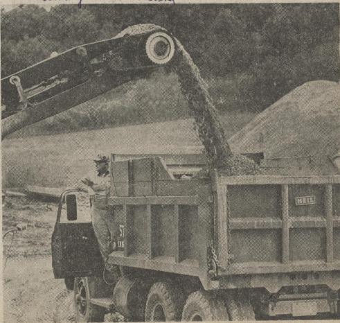
The finished product for use in a variety of construction projects pours into a truck for transport to the site.
