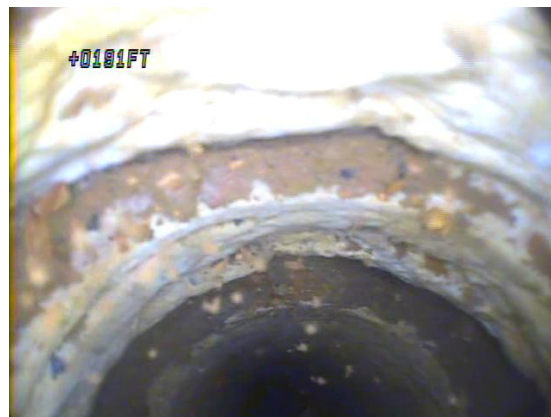
Figure 3: Snapshot from downhole video log of DN-1440 showing hydraulically active fractures at 58 m depth.
