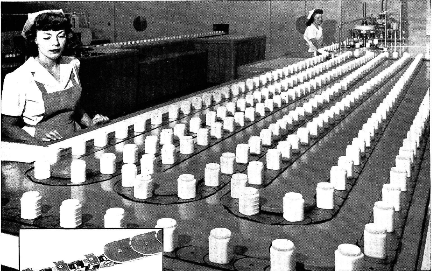
On this Link-Belt universal crescent flat top conveyor chain, jars of baby cream take this irregular path, each always riding separately on its own chain top plate.
