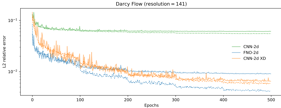
Figure 11.5: Training curves (dotted) and test curves (solid) on Darcy Flow at resolution 141, showing better generalization of XD-operations.
