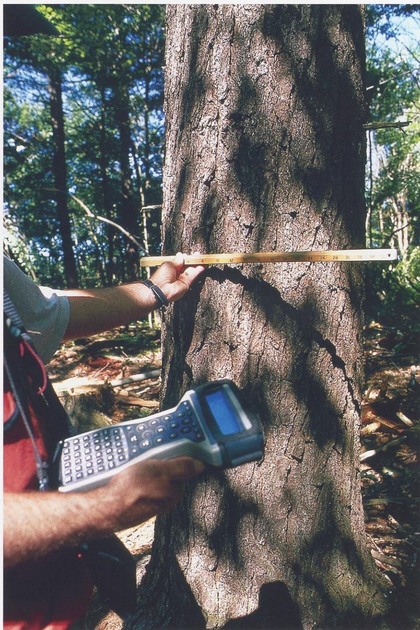
This forester is cruising timber with a data recorder and a Biltmore Stick. The Biltmore Stick is an old tool dating to the middle of the 18th century. The concept is simple: a device that can be used easily in the field to measure trunk diameters and estimate heights of standing trees.
