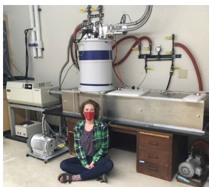
Figure 8.3. Picture of the new MCD installed Feb 2021. An MCD has three main parts, the box that makes circularly polarized light (white, far left), the magnet where your sample sits (also white, middle), and the detector that captures the transmitted light (inside the box, right). In this technique you are essentially measuring the color of a solution in the presence of a magnetic field, at very low temperatures (4.5 K = -269 °C = -452 °F).
