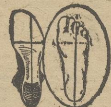
INFLARE—where more of the surface across the ball (A-B) is inside instead of outside the line (C-D).
