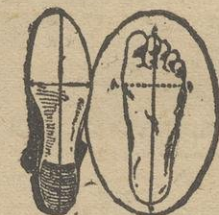
STRAIGHT—where the surface across the ball (A-B) is equal on either side of the line (C-D).
