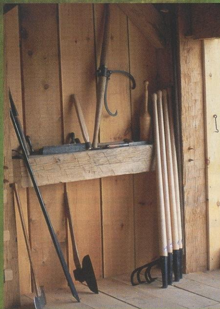
At the Wade House's newest attraction, visitors see how axes, crowbars, log lifters and cant hooks were used to align sawlogs that were cut into timber at sawmills.
