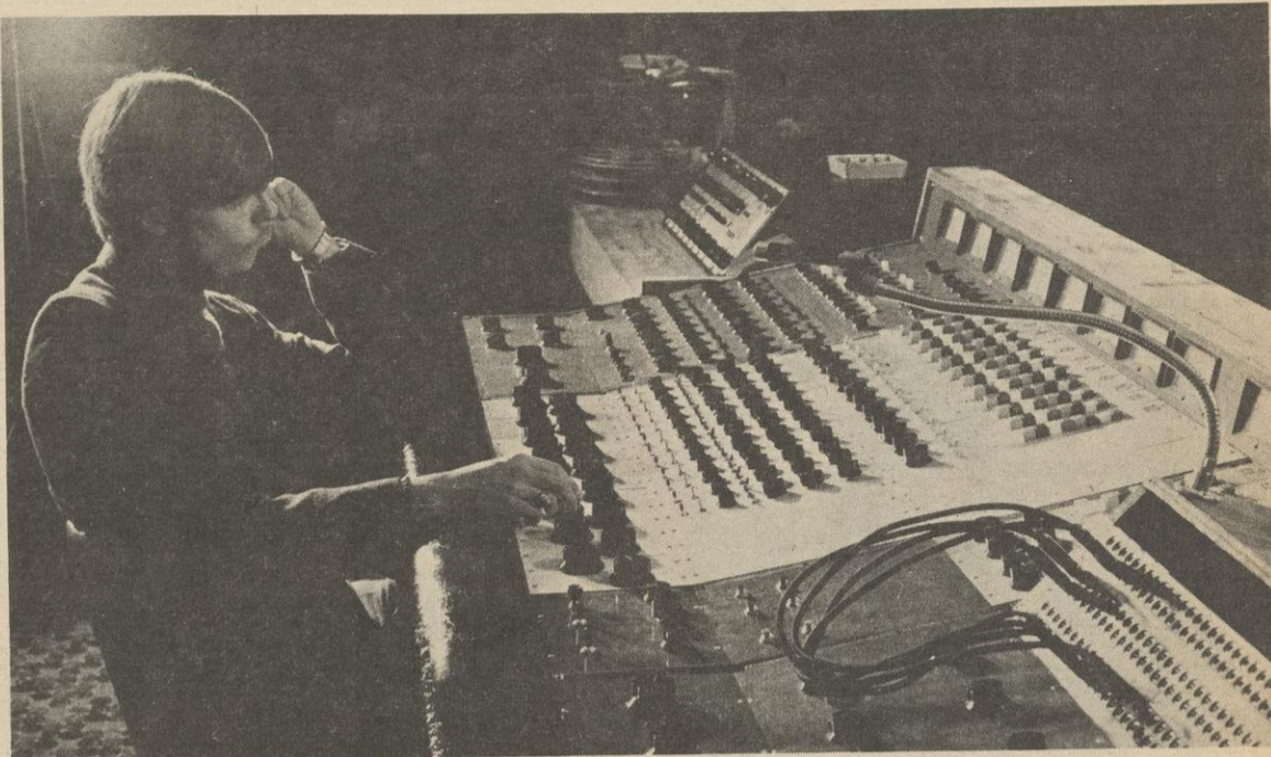
The Full Compass console can handle up to 20 inputs—including 16 microphones or lines, and four echo systems.
