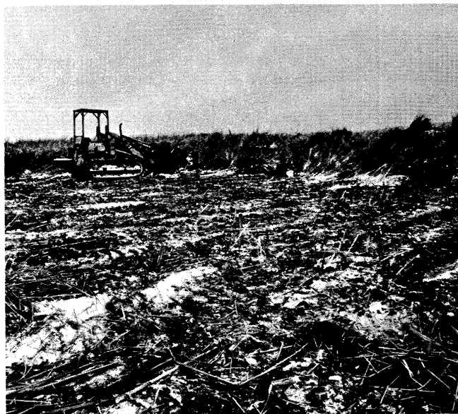
FIGURE 26. John Deere 450 crawler tractor and bucket used to scrape openings (Horicon, 1977).
