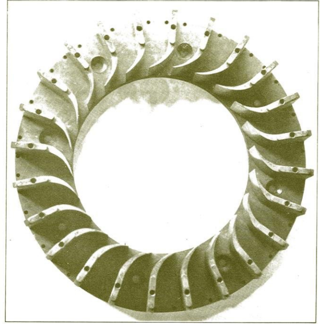
FORMS OF IMPELLER BLADES, EXPERIMENTAL CENTRIFUGAL PUMP
