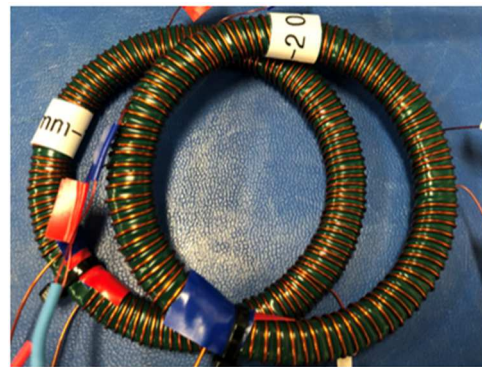
(b) Toroidal core sample with 0.27 mm material
