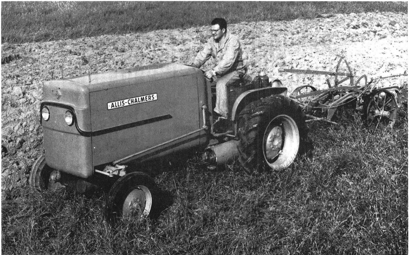
Tractor that is powered by fuel cells.
